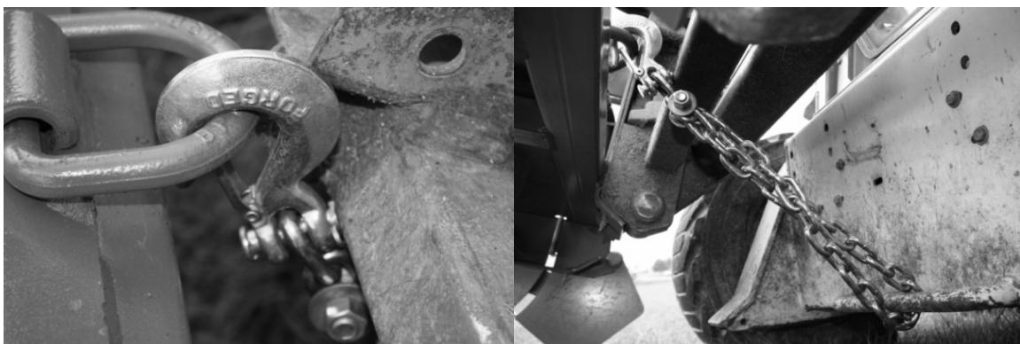
Fig. A. Mower D-ring with safety hook securely attached. Fig. B. Safety chain attached securely to skid steer tie down bar. Safety Chain assembled limiting height not to exceed 18".
